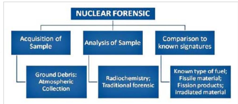
material to the perpetrators? Is this case connected to previous cases? Nuclear Forensics analyzes the nature, use and origin of nuclear materials. Nuclear materials have a "nuclear fingerprint" defined by radioisotopes, isotopic and mass ratios, material age, impurity content, chemical form and physical parameters. Identifying this nuclear fingerprint can help investigators track nuclear materials back to their origin.
